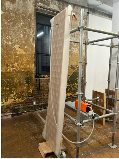
Pressure device , 2022, vacuum bag, vacuum pump, electrical cord, cherry, mahogany, veneer tape, MDF, plywood, netting, hardware
